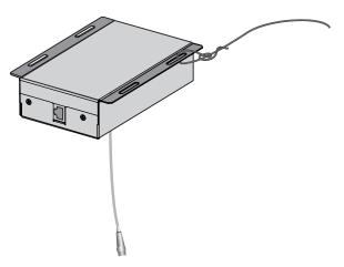
For added safety when removing the ceiling tile at a later time, securely attach the electronics enclosure to the ceiling supports using suitable wire or other hardware appropriate for your ceiling type and in accordance with local regulations. Be sure that the length of wire you use to secure the electronics enclosure is short enough to prevent the enclosure from striking the person removing the ceiling tile.
