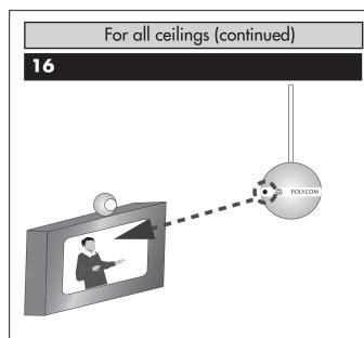
For Polycom SoundStructure C-Series Systems that are being used with a video conferencing system: You must point the dot (located on the band around the middle of the microphone ball) towards the main display.
