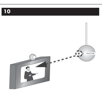
For Polycom HDX: You must point the dot (located on the band around the middle of the microphone ball) towards the main display.
