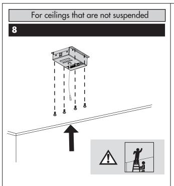
To attach the electronics enclosure, use suitable hardware for your ceiling type. Align the enclosure so that, when the Microphone Array is attached, the dot on the Microphone Array points towards the main display as shown in Step 10 on this page.
