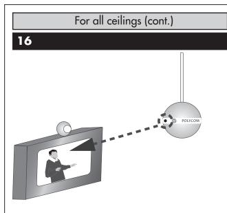
You must point the dot (located on the band around the middle of the microphone ball) towards the main display. 17
